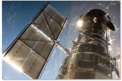
Orbiting high above the Earth, the Hubble Space Telescope has a clear view of the universe free from the blurring and absorbing effects of the atmosphere. In addition to observing visible and near-infrared light, Hubble detects ultraviolet light, which is absorbed by the atmosphere and visible only from space. The telescope has beamed hundreds of thousands of celestial images back to Earth during its time in space.
